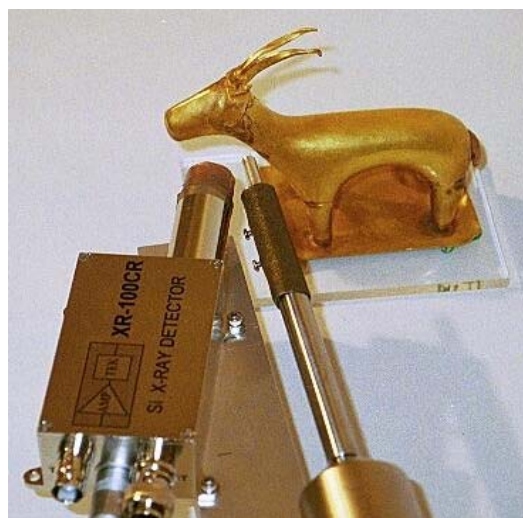
Figure 1. The Gold Ibex Figurine with the Amptek XR100CR X-ray detector and the Photoelectron PRS400 X-ray tube.
